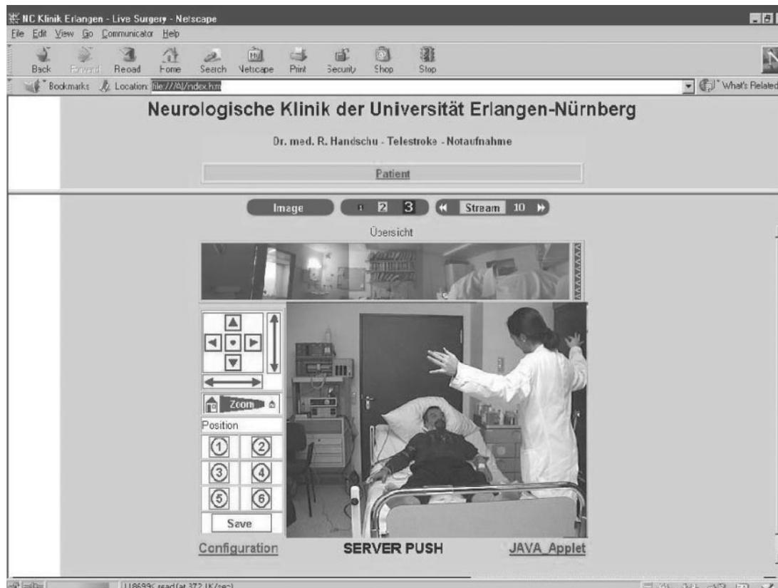
Video examination as seen at the desktop-PC. The video appears in a browser frame. Clicking in the scan view at the top will shift the camera position to that point. At the left side camera position can be operated by mouse click as well as zoom from wide angle to close up. The view shows testing for visual field deficit, where bedside assistance is required.
